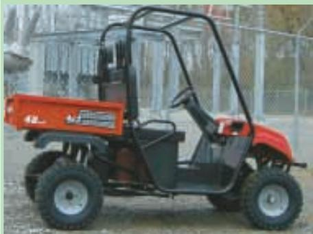
Electric-powered "Chuck Wagon" utility vehicle runs quiet and can handle up to a 400-lb. payload that can be manually dumped.
