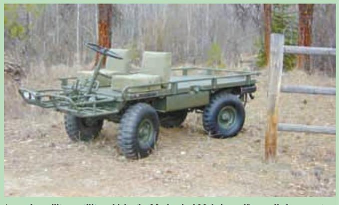
A surplus military utility vehicle, the Mechanical Mule is a self-propelled wagon, tow truck, and walk-behind flatbed all rolled into one.
