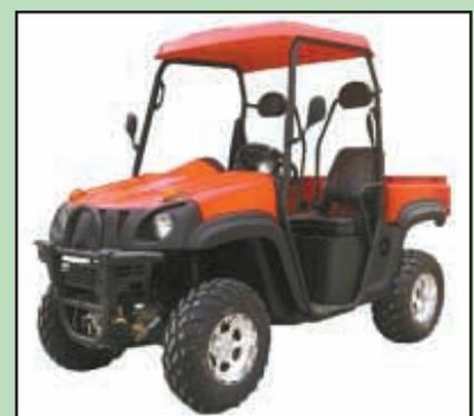
UTV300 Hart cart utility vehicle has a hydraulic dump and gets up to 50 mpg.
