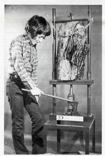
Kids of all ages, from 9 to 90, can operate the Abe Lincoln with one hand, says the manufacturer. Note spreading "dogs" welded to each side of the horizontal wedge-shaped blade at the top of the log.
