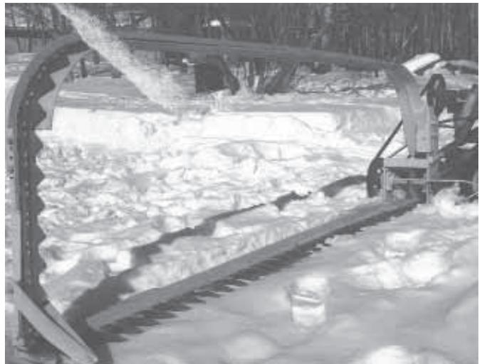
Endless cutterbar consists of knife sections attached to a conveyor chain. The chain of sections slides through a 9-ft. cutterbar from an old Case mower.
