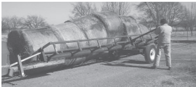
Operator releases all the bales at once by simply flipping a lever.
