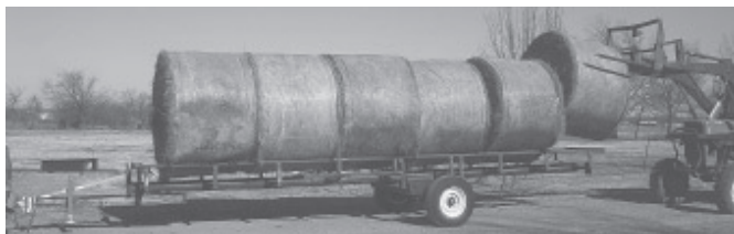
A front-end loader is used to load bales one at a time from the rear, with each bale pushed forward as a new one is loaded.
