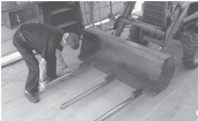
Three 4-ft. removable fingers are made from cold rolled pipe and can easily slide under a standard pallet.
