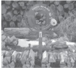
Wood Beaver Twister firewood wrapper is operated by pushing on a foot pedal.
