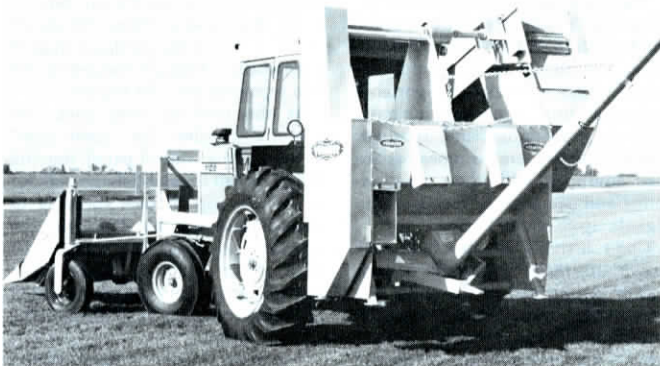
Side view shows rear mounted shelling unit which is carried by tractor's 3 pt. hitch.
