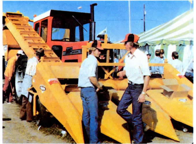
Vermeer will make the new picker available for mounting on several makes of tractors, and with 4 or 6 row heads.
