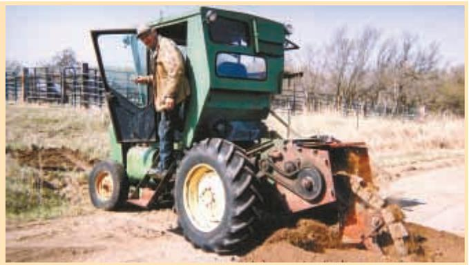
The Ditch Witch attachment on back of combine gets a lot of use running water lines to cattle troughs and underground irrigation.
