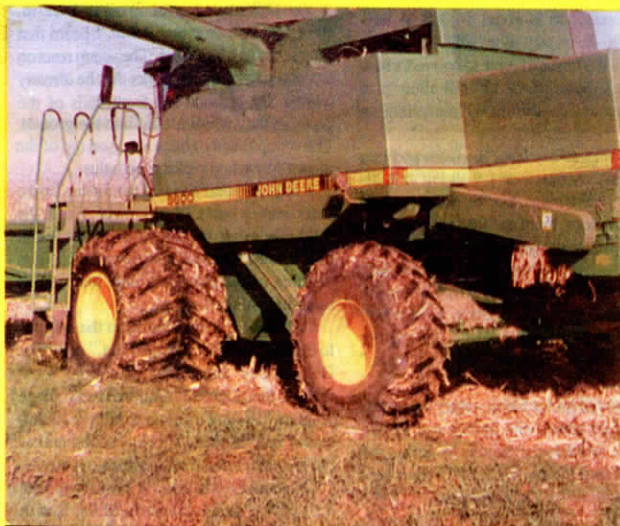
Photo shows "swamp tires" mounted on a 9600 Deere combine owned by Leroy and Gary Fultz, Taylorville, Ill. Farmers who've tried them say the big 50-in. wide tires float over mud rather than squishing it out to the sides.
