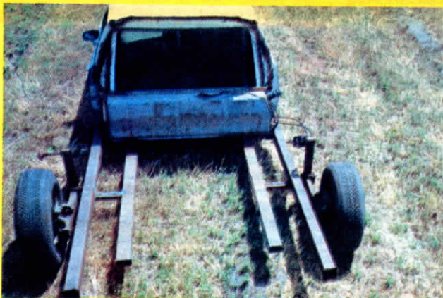
Schlenker cut the rear end off a 1981 Citation to make a bale mover that lets him and his wife haul bales in comfort. Add-on rear bale lift frame is fitted with wheels mounted on pivoting hub assemblies that lower rear end to the ground to load bales.
