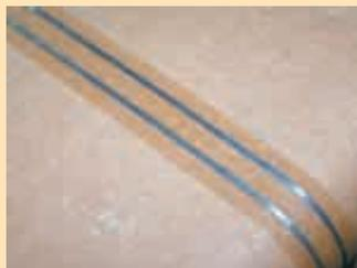
Peel-and-stick electric tape is 1 3/4 in. wide by 1/16 in. thick and encases two aluminum wires. "When a bird's foot touches it, a spark jumps, traveling through the bird's foot," says Mark Ravenelle.
