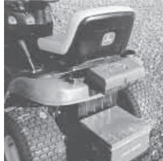
Tin cargo carrier can be mounted or removed in just seconds with brackets that hook to tractor’s frame next to the hitch.
