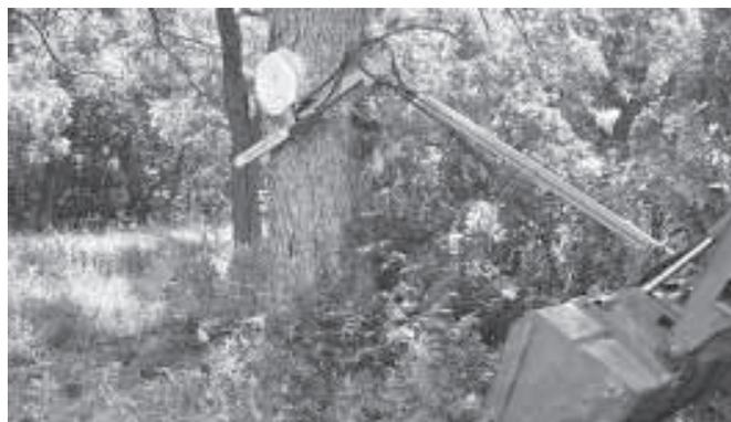
Tree trimmer has an 8-ft. mast and mounts directly to receiver on front-end loader.
