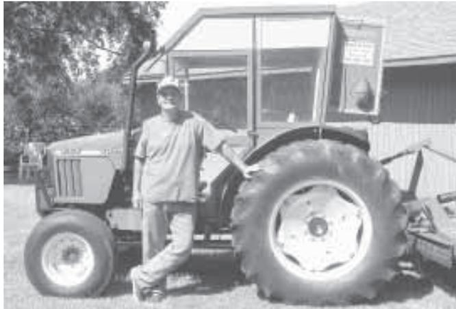
Gary Wear built this cab and evaporative "swamp cooler" for his Deere 5105 tractor.
