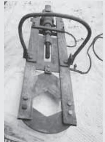
Jim Pardoe automated a long-handled dehorner by mounting the guillotine blades in a frame that's powered by a 1/2-in. drill.
