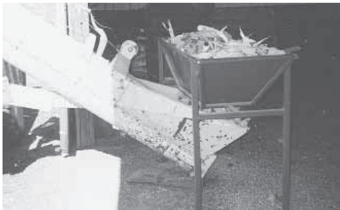
Hopper is about the width of a loader bucket and has an opening at the bottom. It keeps elevator full without overloading it.
