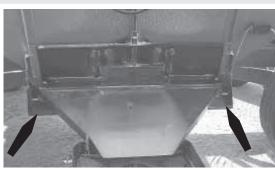
A light sensor is located on each side of wagon chute, sending a light beam across chute which detects when grain stops flowing.
