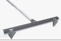
Bolt-on, V-shaped spades can be adjusted for different row spacings.
