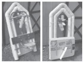
Six direct-driven paddles are located in front, between the pedals (left). A 2-ft. sq. piece of high density styrofoam helps provide flotation
