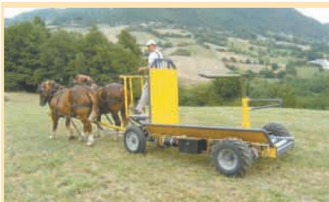
**Horse-powered bale mover uses a mechanical braking system, but ground-powered hydraulics to pick up and handle bales.**
