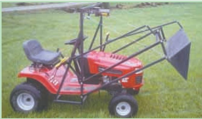
Larry Walton built this front-end loader for his Murray 15 hp riding mower. It can be raised up to 50 in. high and dumped.
