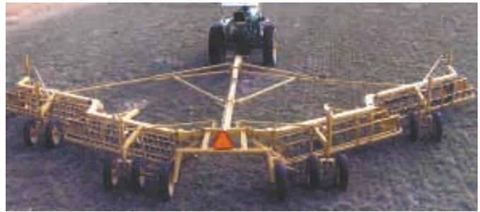
Harold Gleason tore apart four 9-ft. 6-in. New Holland Rolabar rakes to make this 4-ft. bar rake. It folds down to just 13 ft. 6 in. for transport.
