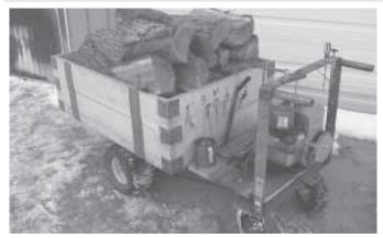
Wheelbarrow is driven by a 5 hp engine. Caster wheels on back allow short turns.
