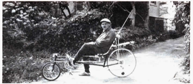
Because the rider pushes back into the seat with his hips, the Avatar 2000 is said to be more power efficient than conventional bicycles.
