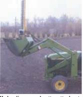
Hydraulic-powered cutter attaches to loader bucket.
