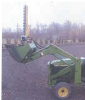
**Hydraulic-powered cutter attaches to loader bucket.**
