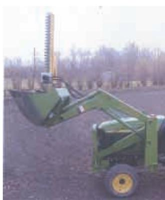
**Hydraulic-powered cutter attaches to loader bucket.**
