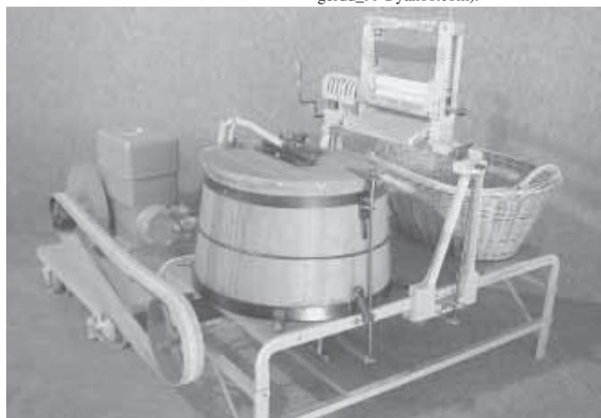
**Manufactured in about 1918, this antique washing machine had a wooden tub and a belt-driven dolly agitator.**
