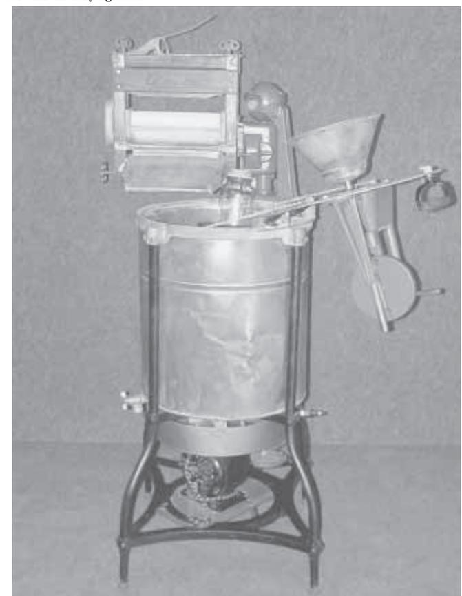
**This machine was manufactured in St. Louis, Mo., about 1920. It had a round copper tub, a cone agitator, and came with either an electric or gas heater.**
