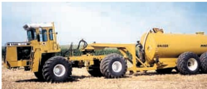
Custom applicator Bob Ward retrofitted a couple of floaters he had been using for herbicide application. Big A 4500 floater (above) carries a 6,000-gal. Balzer tank.
