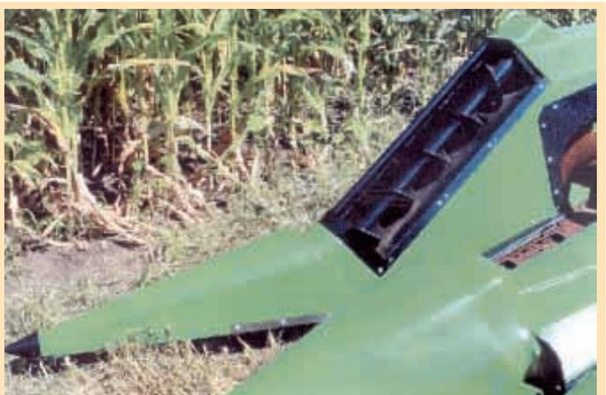
Hydraulically-operated auger kit installs at each end of corn header.
