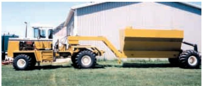
Terra-Gator pulls a 4,200-gal. tank built out of one of the floater's 3,200-gal. tanks. Note application toolbar on back. Unit can go down the road at 40 mph.
