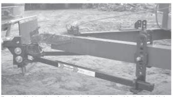
$Equal-i-zer\ hitch is\ easier\ and\ quicker\ to\ hook\ up\ than\ other\ weight\ distributing\ hitches,\ according\ to\ Keith\ Sundling.$
