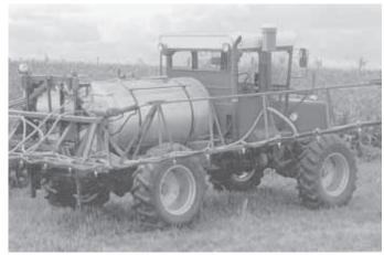
Sprayer has a 500-gal. tank and 3-section, 60-ft. boom on back.
