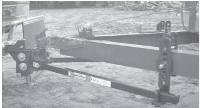
Equal-i-zer hitch is easier and quicker to hook up than other weight distributing hitches, according to Keith Sundling.
