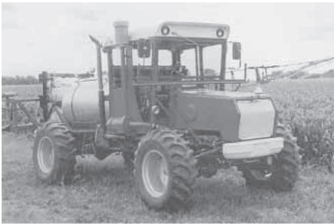
Starting with a 1975 Chevy 1-ton truck chassis, Carl Larson built his own self-propelled sprayer. It's powered by a Perkins diesel engine.
