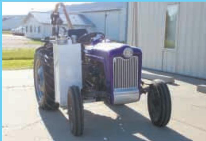
Don Haacke wanted to add a hydraulic posthole auger to his Ford Jubilee, but the tractor's hydraulics were underpowered. So he put a 21 gpm pump on tractor's pto (right) and mounted a 30-gal. hydraulic reservoir on the side of tractor (above).
