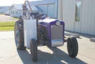
Don Haacke wanted to add a hydraulic posthole auger to his Ford Jubilee, but the tractor's hydraulics were underpowered. So he put a 21 gpm pump on tractor's pto (right) and mounted a 30-gal. hydraulic reservoir on the side of tractor
