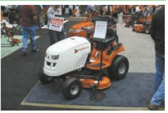
New Allis Chalmers 130 lawn tractor, complete with the old logo and color, has a 23 hp engine with a 42-in, mower deck or a 24 hp engine with a 46-in, deck.
