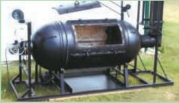
Rotating Turn-A-Nator tumbles the carcass as it burns, using as little as 1/2 gal. of fuel per 100 lbs.
