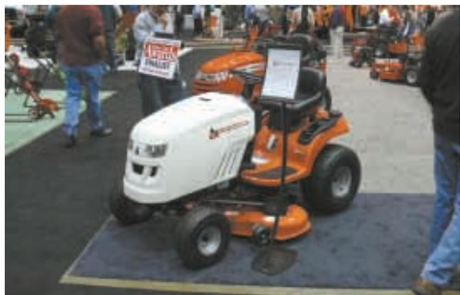
New Allis Chalmers 130 lawn tractor, complete with the old logo and color, has a 23 hp engine with a 42-in. mower deck or a 24 hp engine with a 46-in. deck.
