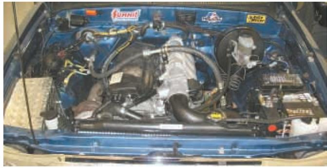
The 5-cyl. engine was a tight fit and required numerous alterations to the pickup's engine compartment.
