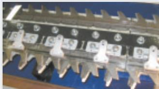
Sickle sections attach to roller chain that runs in a continuous loop.
