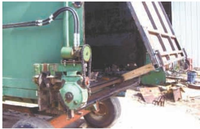
They reversed the box to put the opening in back and built a metal door. They also added the motor from an old fertilizer gravity box auger to drive the apron.
