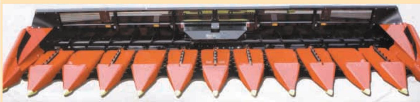
Geringhoff MultiCrop header is equipped with vertical gathering chains in middle of snouts to improve crop flow into auger.
