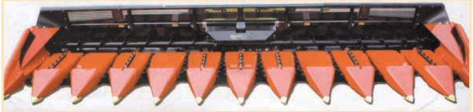
Geringhoff MultiCrop header is equipped with vertical gathering chains in middle of snouts to improve crop flow into auger.
