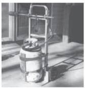
Mounting propane tank and blow torch to hand cart makes burning brush and weeds a much easier job.
