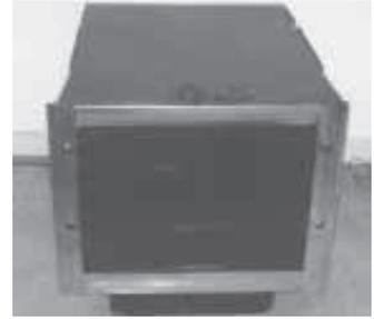
Low-cost electric heater was made from a junked electric cook stove and the radiator off an old pickup.
