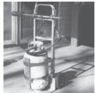
Mounting propane tank and blow torch to hand cart makes burning brush and weeds a much easier job.
