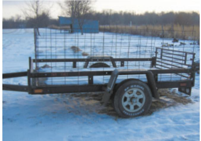
Trailer's sides and front are formed by lengths of cattle panel inside 1-ft. high channel iron sides.
