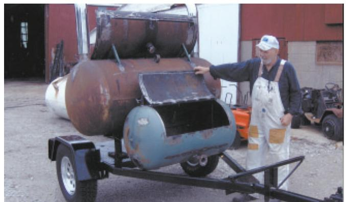
Gene Boehler made this smoker from a used 250-gal. anhydrous ammonia tank. The fire is contained in a 100-gal. tank mounted on front.
