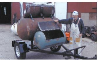
Gene Boehler made this smoker from a used 250-gal. anhydrous ammonia tank. The fire is contained in a 100-gal. tank mounted on front.
