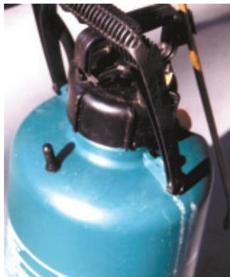
**Jamieson drilled a hole in top of 2 1/2-gal. spray tank and snapped a valve stem into place. When tank needs more air, he pumps it up with a portable compressor.**
