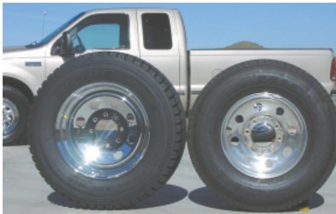
**Replacement wheels allow use of commercial-duty tires on 3/4 and 1-ton pickups.**
