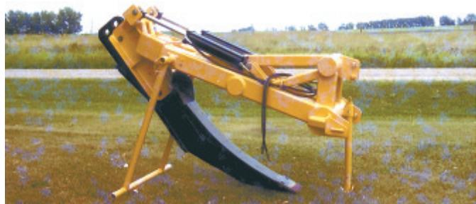
**Janssen's big 3-pt. ripper has a slightly curved shank to bring ribbons of clay subsoil up to the surface. Shank angle can be adjusted on-the-go by extending or retracting a pair of hydraulic cylinders.**
