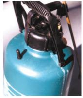
Jamieson drilled a hole in top of 2 1/2-gal. spray tank and snapped a valve stem into place. When tank needs more air, he pumps it up with a portable compressor.
