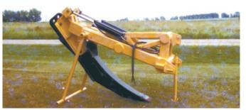
Janssen's big 3-pt. ripper has a slightly curved shank to bring ribbons of clay subsoil up to the surface. Shank angle can be adjusted on-the-go by extending or retracting a pair of hydraulic cylinders.
