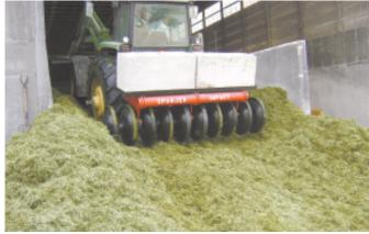
Wheel rims sink up to 6 in. and bring loose material up, forcing air out of silage.
