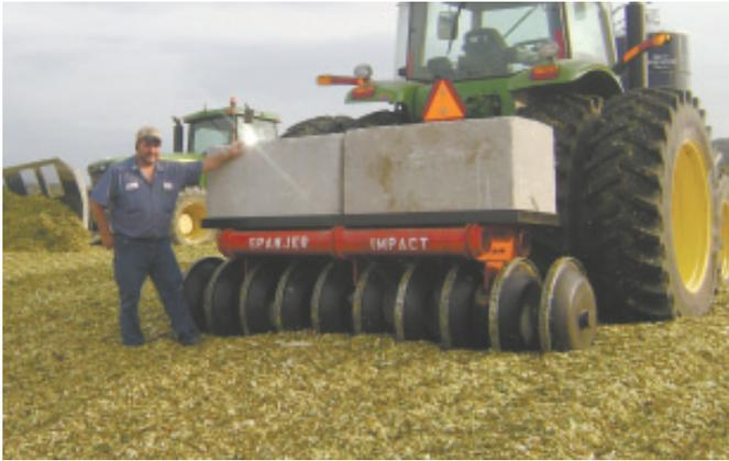
Silage Roller's narrow wheels are custom made for each customer's operation.
