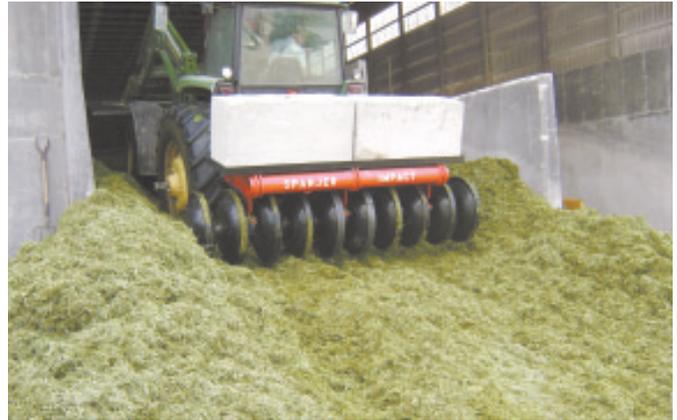
Wheel rims sink up to 6 in. and bring loose material up, forcing air out of silage.
