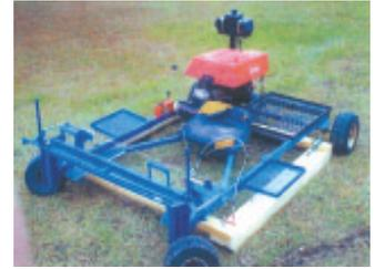
Pickerstraddles 4-ft. wide asparagus rows. Driver picks asparagus and puts it in expanded metal trays on both sides of rig.
