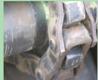
Power Tooth Sprockets have wider spaces between teeth. The design allows more teeth to be engaged at the same time.
