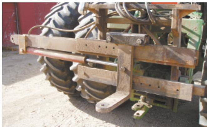
Hydraulic-controlled, 3-pt. mounted drawbar moves 15 in. from side to side.
