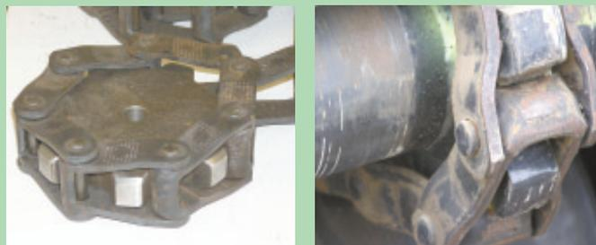
Power Tooth Sprockets have wider spaces between teeth. The design allows more teeth to be engaged at the same time.
