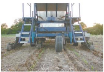
Prototype makes four trenches per pass, with adjustable spacing from 10 to 40 in.
