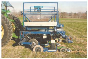
Poultry litter falls from applicator into shallow trenches made by 18-in. coulters, and is then covered by two sets of wheels.
