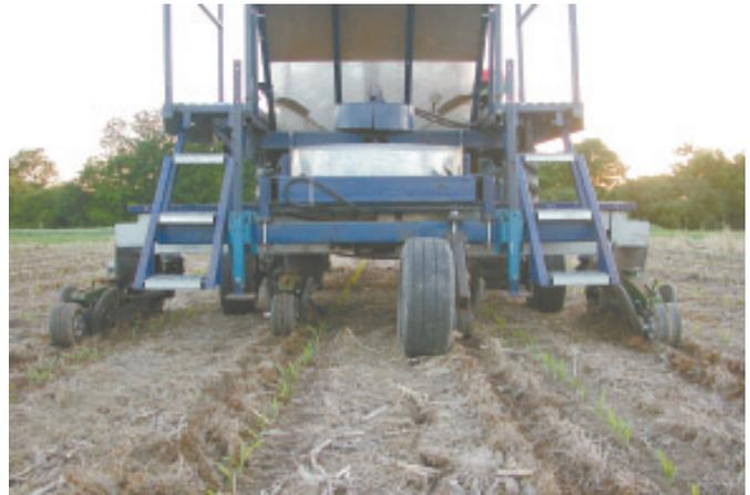
Prototype makes four trenches per pass, with adjustable spacing from 10 to 40 in.
